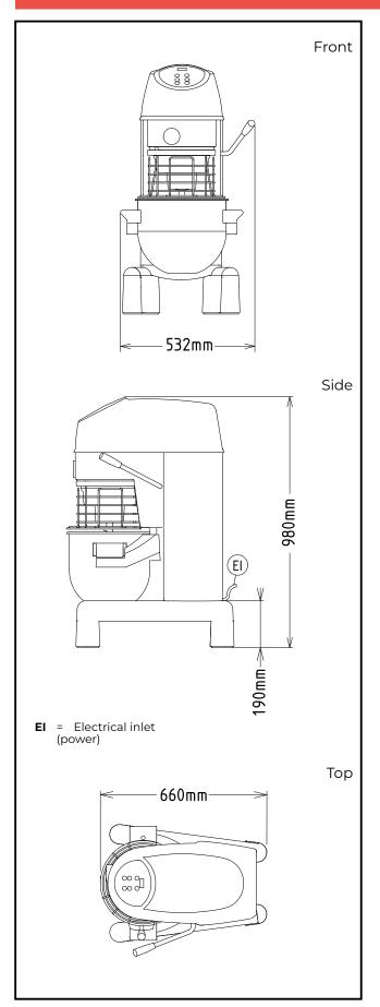
Electric Supply voltage: 200-240 V/1N ph/50/60 Hz Electrical power, max: 1.01 kW **Total Watts:** 1.01 kW Capacity: Performance (up to): 6 kg/Cycle Capacity: 20 litres Key Information: External dimensions, Width: 521 mm External dimensions, 685 mm Depth: External dimensions, Height: 980 mm **Shipping weight:** 87 kg Net weight (kg): 76 **Cold water paste:** 6 kg with Spiral hook
